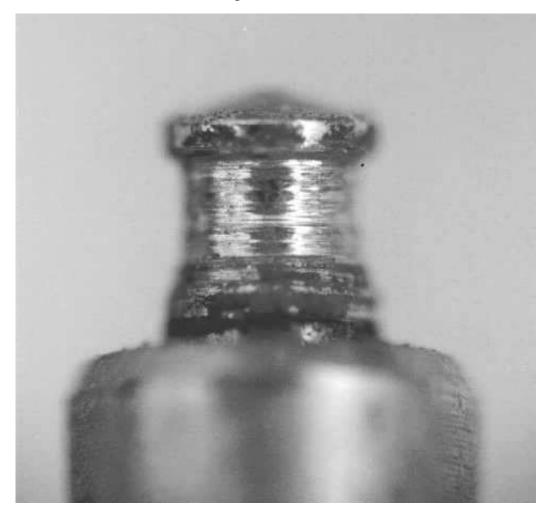
The pivot would have a considerably smaller diameter after polishing, so the bushing would need to be replaced with a bushing that has a smaller hole.
