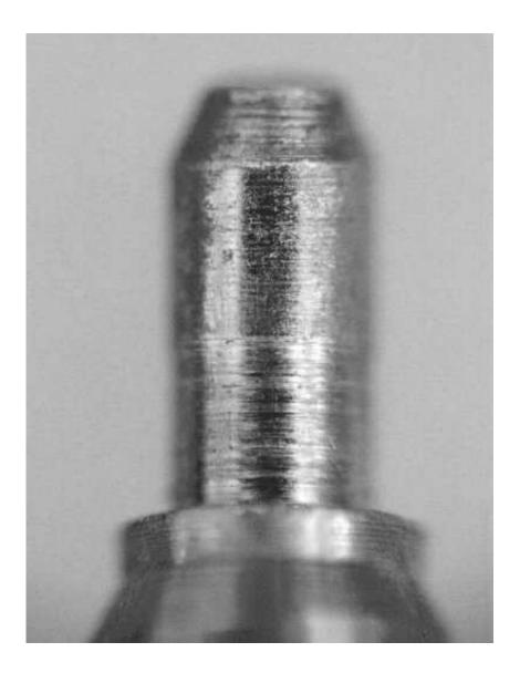
This kind of wear is obvious to the eye, even without a loupe. The cause is rust: once oxidation begins, particles of rust float in the lubricant, acting as an abrasive and causing scoring of the pivot when the rust becomes embedded in the brass bushing surface.
