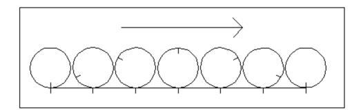
If you draw a line to trace the path of the point as the circle rotates, the result is called a Cycloidal Curve.
