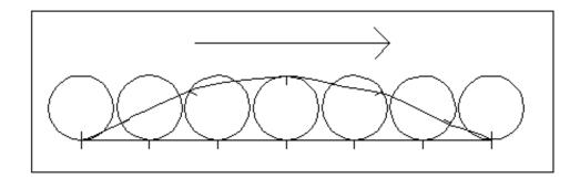
This curve is inaccurate in its shape because of the way I created these drawings, so below is a much more accurate Cycloidal Curve, generated in a chart of the horizontal and vertical coordinates of the path of the point as the circle rotates. The chart is used here to create the graph below (with Rotation in Degrees on the X axis and Displacement in Inches on the Y axis).
