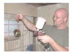
This clock dial pan and bezel have been cleaned and are ready to be polished and lacquered.
