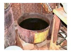
The acid is removed by rinsing thoroughly in water. The part is dipped into a buffer like sodium bicarbonate solution and then rinsed again thoroughly in water. (A mild base like ammonia solution could also be used in place of the buffer). Apply stripper with a paintbrush and leave for five minutes. Rinse again thoroughly in water.
