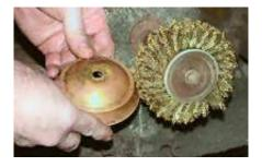
Polishing takes place in two steps. First polish with a cotton wheel using tripoli (a fine abrasive compound). Clean off the residue with lacquer thinner (other solvents can also be used).
